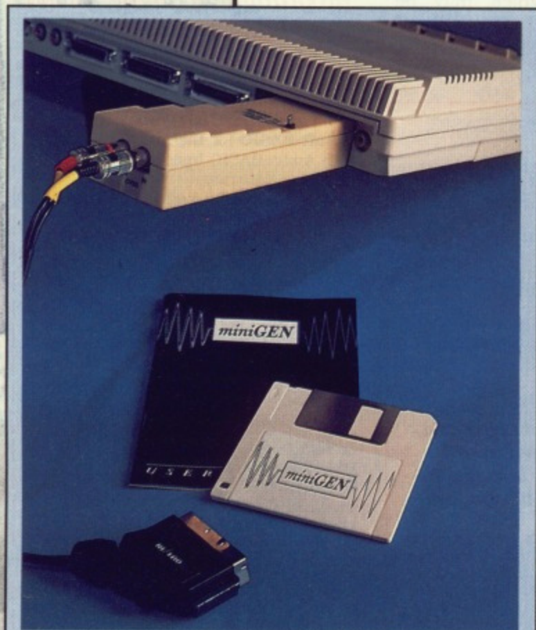
■ The miniGEN itself looks very similar to the Amiga's modulator case but the noticeable differences are that it's been moulded in a shade of light yellow and has a small toggle switch on the top labeled 'Mixed', 'Graphics' & 'Picture'. At the back are two phono sockets, one marked 'Video Out' and the other 'Video In'.
