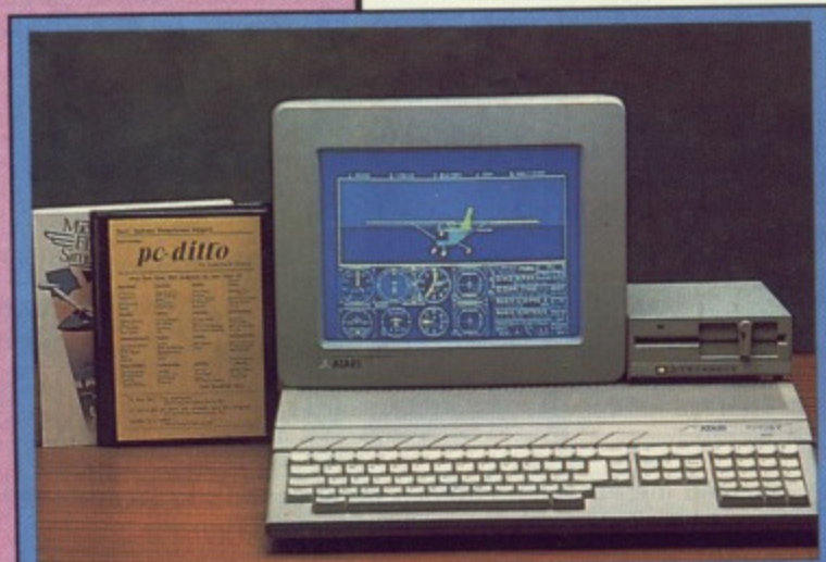
■ PC Ditto up and running MicroSoft's Flight Simulator, the classic test of PC compatibility, albeit rather slowly. The extra 5.25" drive is made by Triangle (available through Power Computing, £115) and gives access to most PC software.
